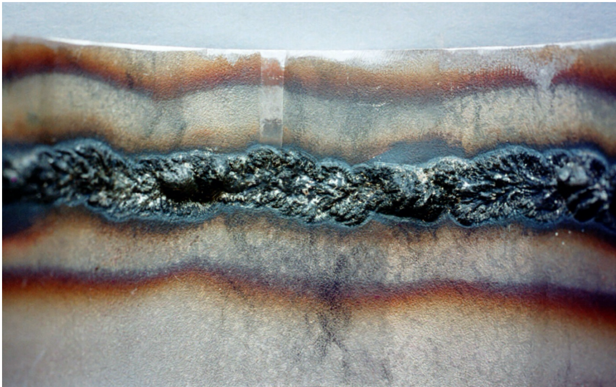
This photograph shows the root side of a weld that was made using GTAW open root with the root side exposed to air. Note the coarse, irregular surface.
